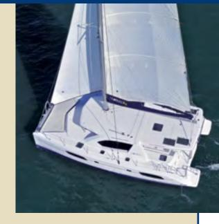
The most significant modification on the Leopard 44 is the addition of the open forward cockpit with direct access from the saloon. Unique to production catamarans this feature offers increased visibility, ventilation, and a significant new approach on adding increased living space in an ergonomic and safe design feature.
