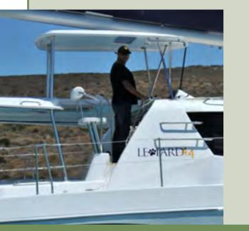
First introduced on the popular Leopard 46, and continued with each model since, the Leopard 44 features a raised helm station covered by a hardtop bimini. With direct access from the cockpit and weather deck and all lines leading aft, the helm station offers a central and secure location for sail and yacht control.
